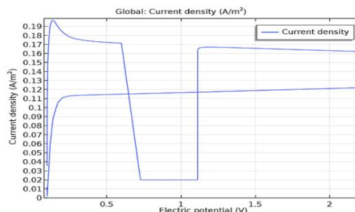
Fig. 10. Cyclic voltammetry current vs electrolyte potential.
