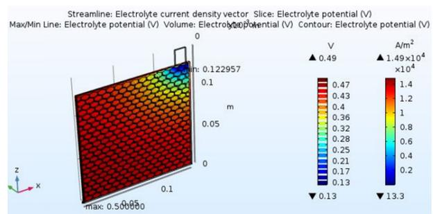
Fig. 6. Heat production during electrode current density and electrolyte potential of hexagon plate.
