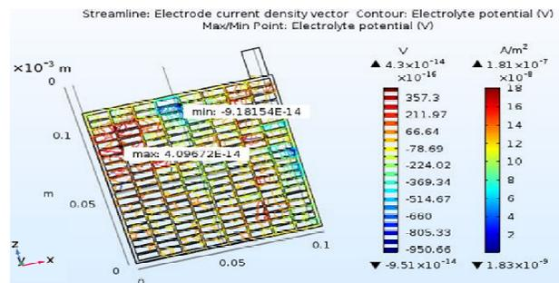
Fig. 5. Electrode current density and electrolyte potential of rectangular plate.
