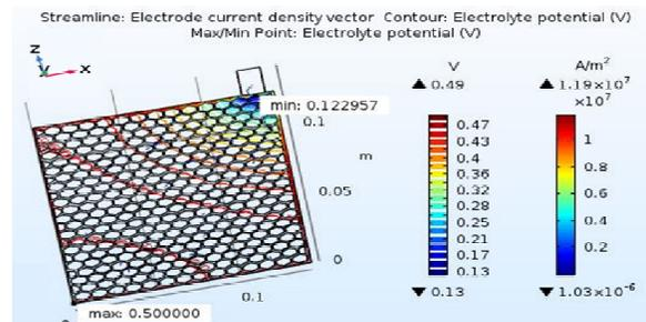
Fig. 4. Electrode current density and electrolyte potential of hexagon plate.
